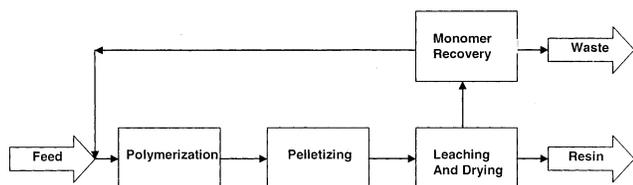
**Figure 1.** Block diagram of a conventional nylon-6 polymerization process.
