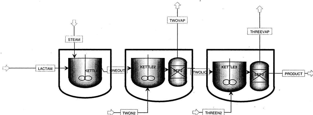
**Figure 9.** Three-reactor nylon-6 manufacturing process. Lactam and water are fed to the first multiphase kettle, while inert gas flow devolatilizes the second and third vessels.
