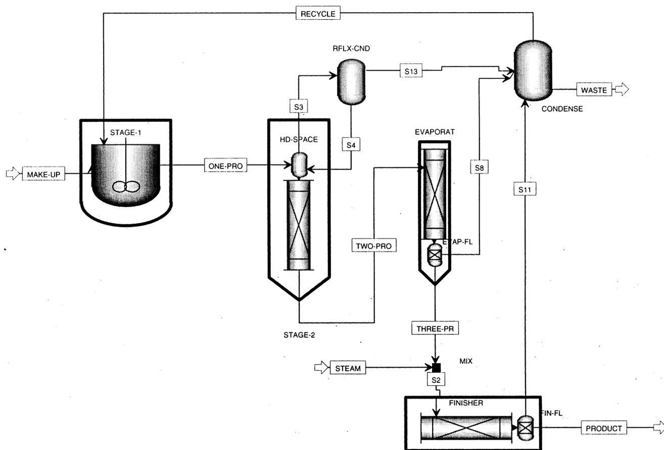
**Figure 8.** Four-reactor nylon-6 manufacturing process. Most of the monomer conversion takes place in the first two reactors, while the molecular weight buildup occurs in the third and fourth reactors. The second vessel has a reflux condenser, while the entire train has a condenser to recycle the unreacted monomer.
