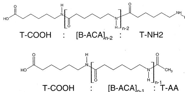
**Figure 2.** Nylon-6 molecules of degree of polymerization  $n$  existing as two types: unterminated (above) and terminated by AA (below). B-ACA represents nylon-6 repeat segments, T-NH<sub>2</sub> represents amine end groups, T-COOH represents carboxylic acid end groups, and T-AA represents AA end groups.
